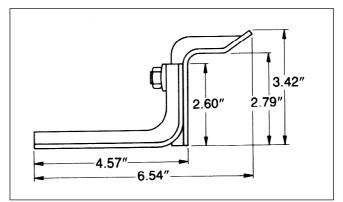
**710894 Adjust-A-Stop** — Adjustable stop for doors 2-3/4" to 4-1/4" in thickness. Recessed bolt head protects door finish. Lag bolts recommended for mounting. Heavy, 10-gauge, zinc-plated steel. Also available white vinyl-coated. (710899)
