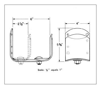
**651403** Adjustable Door Guide or Stop — Adjusts for sliding doors from 2-1/2" to 6-inches thick. Twopiece, 8-gauge, galvanized steel construction with 1/2 - 13 zinc-plated carriage bolt, washer and nut. Curved surfacce forms natural "lead-in" for door, provides rigid assembly when clamping bolt is tightly drawn and keeps mounting bolts or nails from interfering with door movement. Packed, bulk, unassembled. Weigt 3 lbs. each.
