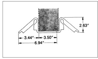
**710950** — Made of heavy zinc-plated steel with rounded corners for maximum protection against tire and livestock injury. Two required for center of double-leaf doors. Also 711228 Center Stop and Hold Down package. Designed to stop and give positive hold down protection against wind lifting doors out of guides. When used with 710950 Guide Half, makes complete door guide and stop package. Comes in plastic bag with bolt and nut.
