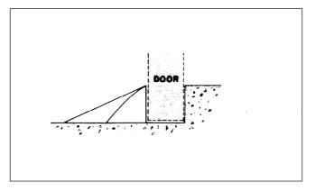
**652901 Center Door Guides** — Hold sliding doors in place. Beveled, cast-iron shape protects tires. Eccentric washers rotate to adjust for door thickness. Size  $1-3/4" \times 4" \times 9-1/2"$ . Gray finish. Packed bulk, less fasteners. Weight 2.7 lbs. each.
