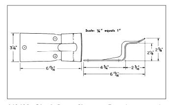
**643411 Giant Door Stop** — For doors up to 2-inches thick. Made of 10-gauge, pressed steel. Zinc-plated. Packed bulk. Weight 1.1 lb. each.
