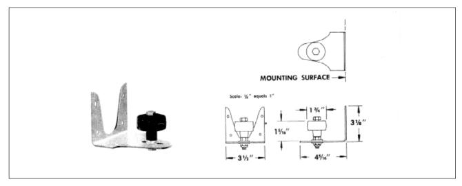
**710590 Universal Stay Roller** — Can be screwed to building wall or mounted in concrete floor by inverting the angle so that the bracket legs act as an anchor in the concrete. Adjusts for doors 1-5/8" to 2-3/4" thick. Mounting angle is made of 12-gauge zinc-plated steel. Wheel is black DuPont Delrin plastic. Packed bulk. Weight .9 lb. each.
