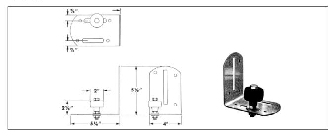
**650706 Off-Set Stay Roller Assembly** — Offset slots allows the black DuPont Delrin Plastic wheel to be at edge of bracket to contain doors which have a small overlap on the door jamb in the closed position. Adjustable for doors 3/4" to 2-1/4" thick. Mounts with lag bolts, screws or nails (not included). Angle can be inverted for anchor in concrete. Mounting angle is 8-ga. zinc-plated steel. Packed bulk. Weight 1.9 lbs. each.
